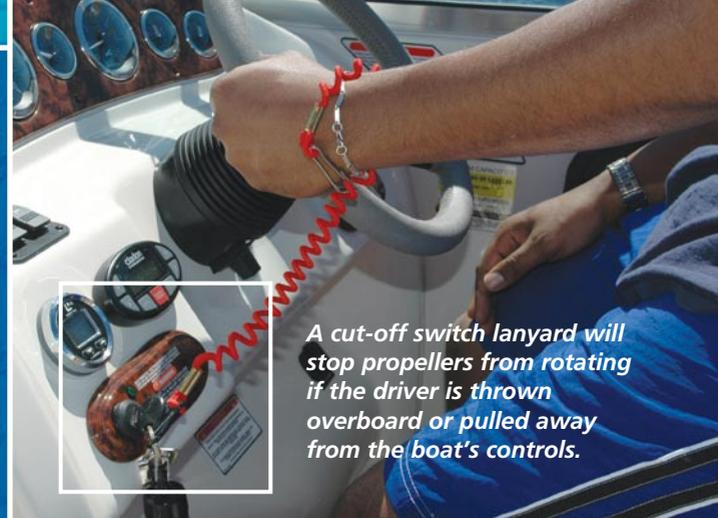
*A cut-off switch lanyard will stop propellers from rotating if the driver is thrown overboard or pulled away from the boat's controls.*
