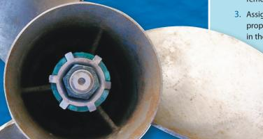
A typical three-blade propeller running at 3,200 rpm can inflict 160 impacts in one second.
